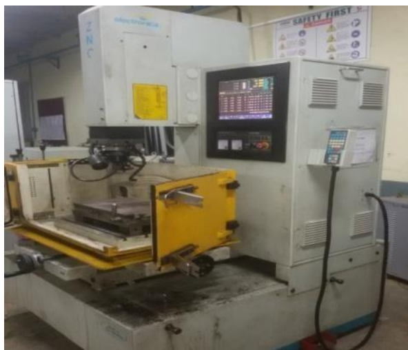
Fig. 2 Electrapuls PS 50 ZNC electrical discharge machine
