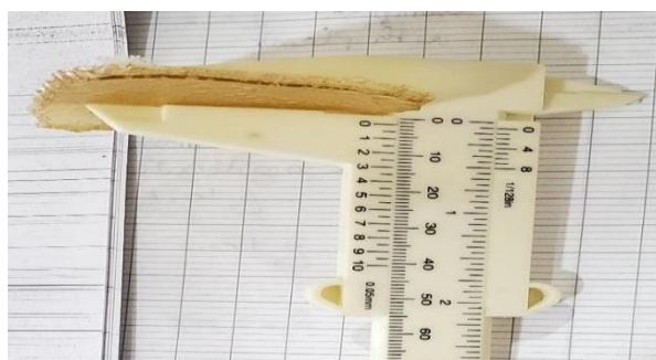
Figure 1: Thickness measurement for starch–gelatin bioplastics typically
