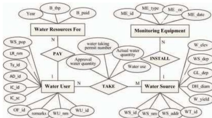
Figure 3. The entity-relationship diagram of rural water resources information management system
