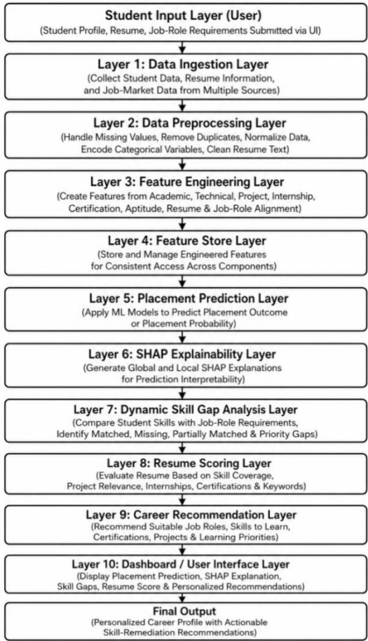
Figure 1. System architecture of the proposed hybrid explainable AI framework for student placement prediction and personalized skill gap remediation.
